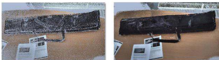
Figure 5: Carry bag scanned with a Freestyle3D. Data without using best-point filter (left) and with the filter (right).
